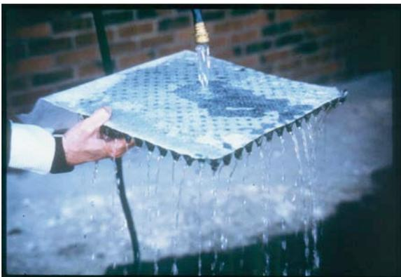
Geotextile filter and 3-dimensional plastic drainage core
