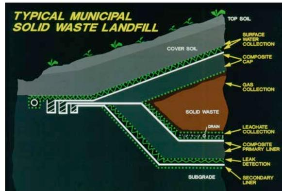
There are many ways that geomembranes and GCLs have been incorporated into environmental protection barrier systems, including:
